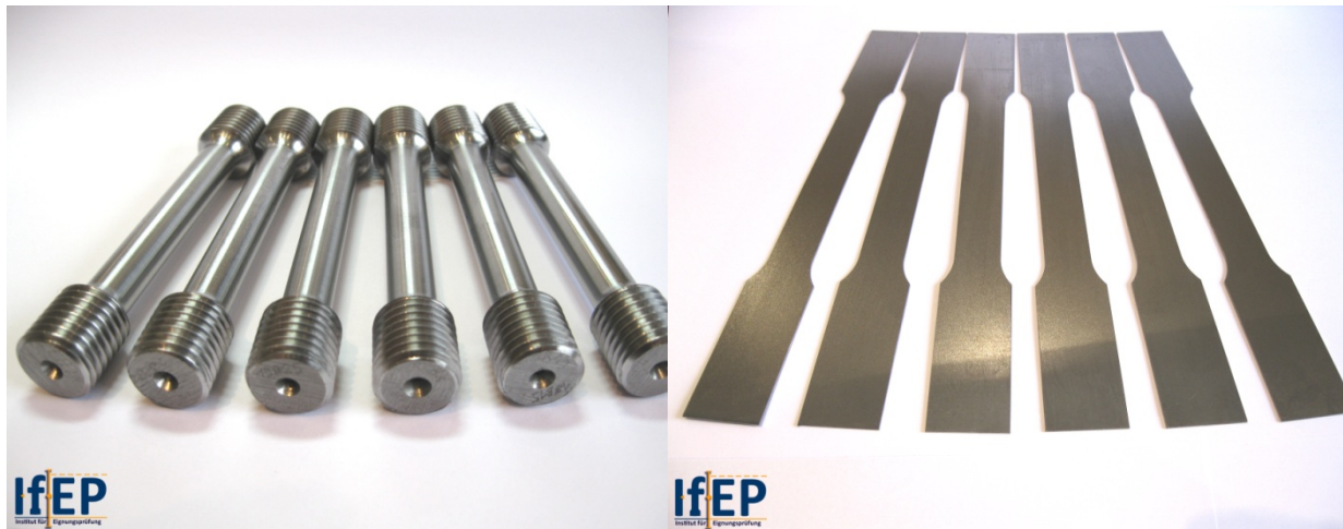
Round bar test specimens
